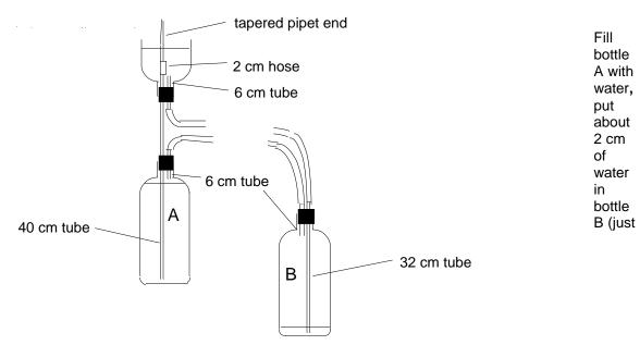
enough to get the water level above the bottom of the long glass tube) and secure all stoppers. To start the fountain, place bottle A on the table and bottle B on the floor, then fill the top funnel with water. Within a few seconds, the fountain will begin spurting up out of the tapered pipet end. To control the rate of flow, adjust the relative heights of the two bottles.
