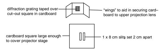
Tape the large square of cardboard over the projector stage. Tape the diffraction grating over the hole in the small piece of cardboard with wings and then tape this assembly over the upper projection lens.
