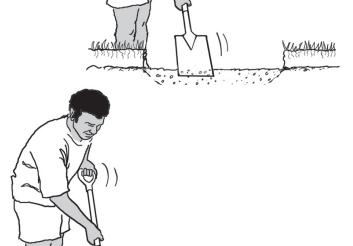
If you have to fill-in deep areas, fill with rock — or old blocks or pieces of concrete. Cover with sand and compact it all down to make it hard and level.
