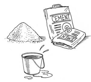
Mortar is made from 4 parts sand and 1 part cement mixed with water.
