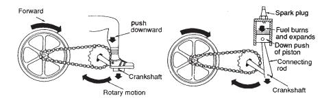
The engine crankshaft is then connected to what the engine is driving – a wheel, propeller, cutting blades.
