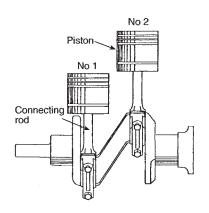
Two-cylinder engines are common for outboards and motor bikes
