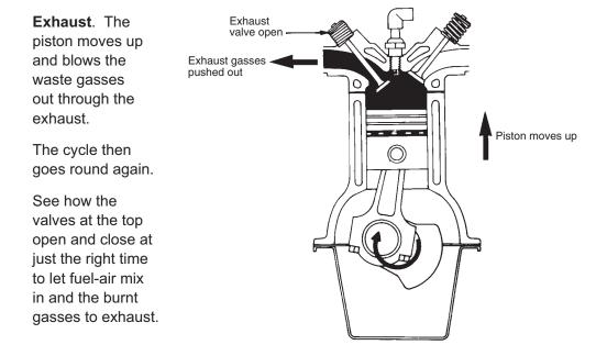
A flywheel fixed on the end of the crankshaft keeps the engine turning during the exhaust and intake strokes.
