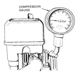
The pressure should be between 60 and 100psi (pounds per square inch) for a 2-stroke and up to 150psi for a 4-stroke. On engines with more than one cylinder, they should have compression within about 10-15% of each other.
