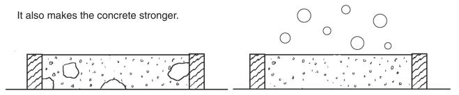
Compact as soon as the concrete is poured and while it is workable.
