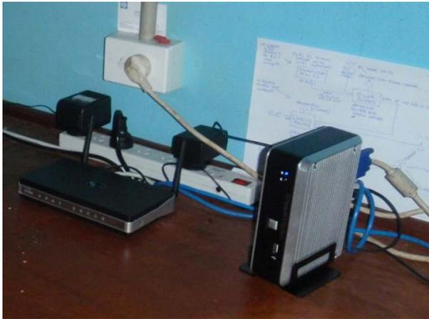
On the left is an example of a low cost, low power fanless PC computer costing less than USD 800, which consumes only 10-15W of power. Ideally, two network adapters (NICs) should be used, one which can be connected to the Internet (optional) and one with the local network (LAN) with the wireless access point(s). Depending on local sunshine/insolation, one 130W solar panel may be sufficient to support this device 24 hours per day.
