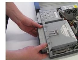
Remove the CD drive from the case by disconnecting the data and power cables at the back by pulling it out.
