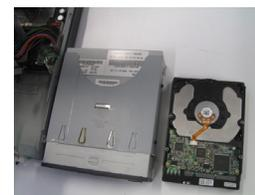
At this point, both the CD drive and the hard drive should have been removed from the computer case.
