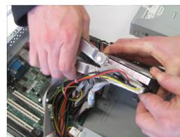
Remove the hard drive from the case by disconnecting the data and power cables from the back and lifting it out.
