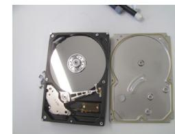
Remove the circuit board and the screw indicated to access the disks and remove the magnet.
