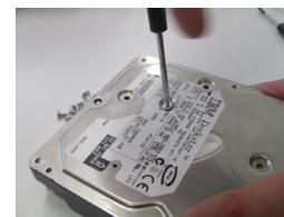
Remove the screws on the top of the bearing, take off the bearing and remove the bearing.
