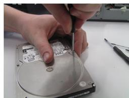
Remove the screws from the back of the hard drive to open it up.
