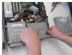
Remove the metal cover that is obscuring the hard drive. Be careful of sharp edges.
