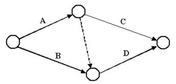
The dummy activity (shown by the dotted line) is needed in the AOA network to show the predecessors correctly, i.e. that D depends on both A and B, but C depends only on A. AOA networks often need several dummy activities. AON networks do not need dummy activities.
