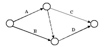
The **Dummy Activity** (shown by the dotted line) is needed in the AOA network to show the predecessors correctly, i.e. that D depends on both A and B, but C depends only on A. AOA networks often need several dummy activities. AON networks do not need dummy activities.
