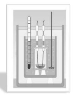
An experiment was carried out to determine a value for the enthalpy of combustion of liquid methylbenzene using the apparatus shown in the diagram.
