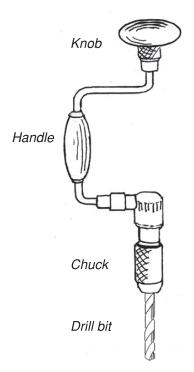
A drill **bit** cuts into the timber as it is turned.
